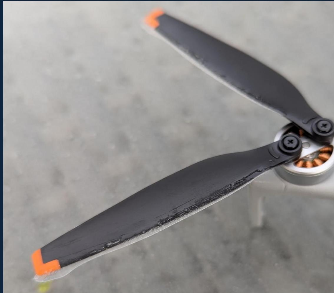
Icing on a drone propeller
